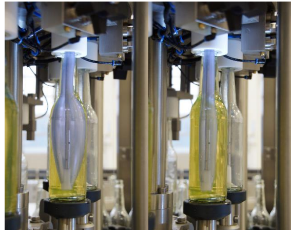
Bottling using the balloon-style method
